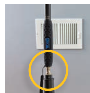
The EXP-64 can be mounted on tripods for longer term analysis of airflow from wall or ceiling vents
