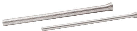
SPRING TYPE TUBE BENDERS • For soft copper and aluminum tubing • Special spring steel with zinc finish • Hand bend tubing to any shape without collapsing walls End bell design for quick removal of tubing
