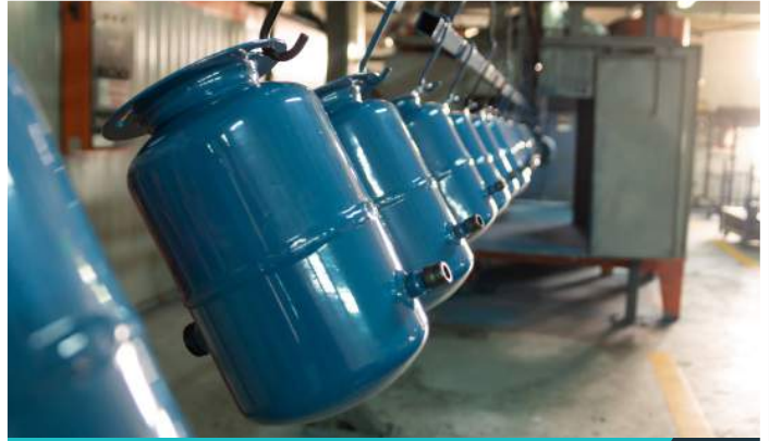
full automatic powder coated paint line tam otomatik raylı toz boya hattı
