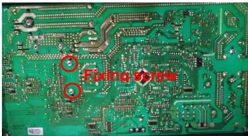
Heat radiation problem easily happened while the screw is not fixed tightly.
